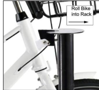
Pull back on bike to confirm it is secured to rack.
